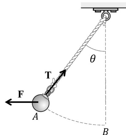
b) If the ball is released ( $F = 0$ ), what will be the speed of the ball at point B?
