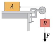
c) After the boxes start moving, find the magnitude of the pulling force  $|\vec{F}|$  required to make the boxes move at constant speed.
