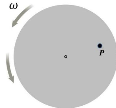
$$\omega = 120 \text{ rev/min} = 12.56 \text{ rad/s}$$
