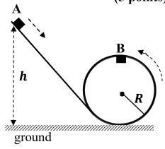
**P4.** A box with mass m = 450 g is sliding on a frictionless track from point **A** to point **B** in t = 8 s while its speed is increased from  $v_A = 1$  m/s to  $v_B = 4$  m/s as shown in figure.
